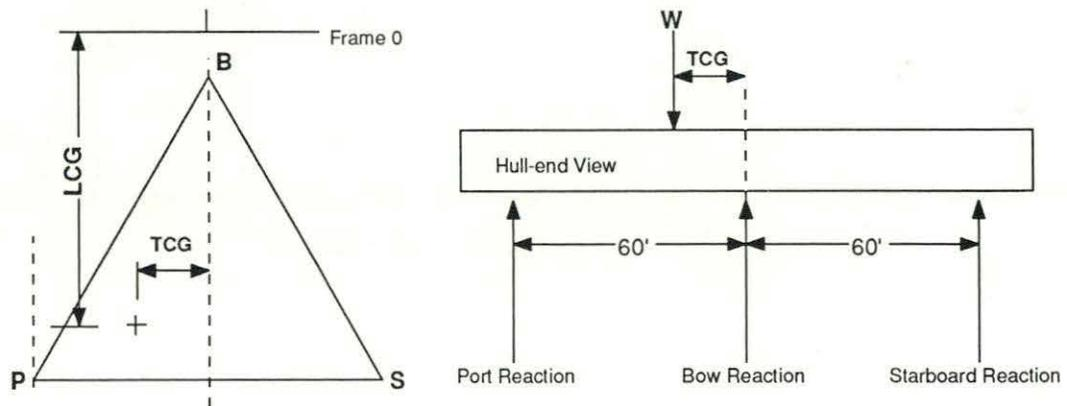
Taking moments about the port leg results in the following equation for the reaction in the starboard leg:
